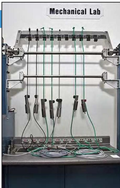
*Continuous, automated flex testing by an articulated arm checks for signal integrity loss.*
